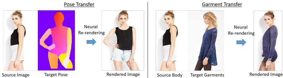
Fig. 1. Given an image of a person, our neural re-rendering approach allows synthesis of images of the person in different poses, or with different clothing obtained from another reference image.
