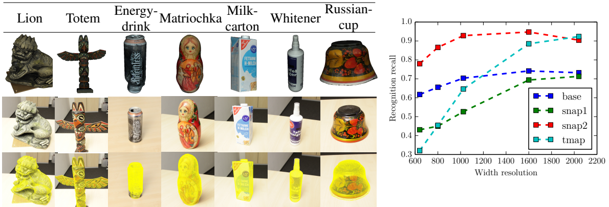
Figure 3: (Left) Models that are considered for evaluations. The first row shows the 7 acquired CAD models. The second row shows the images of the real objects of the corresponding models. The third row shows result of 6DOF recognition where mesh from the CAD models are reprojected on to the 2D images using the extrinsics found. Note that the images are zoomed towards the model for better visualization. (Right) Comparison of recognition recall of our methods with the existing base whose trained model is obtained by the manual way of taking pictures, segmenting and performing SFM.
